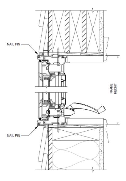
PROVIDE A CONTINUES BEAD OF SEALANT BEHIND THE NAILING FIN BEFORE SETTING THE UNIT IN PLACE AND SEAL FIN WITH WATER PROOF TAPE
