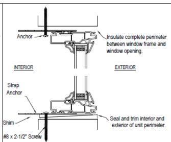
1.) Check rough opening to ensure that the window unit will fit. The rough opening should be 1/4" to 1/2" larger than the window, both horizontally and vertically.
