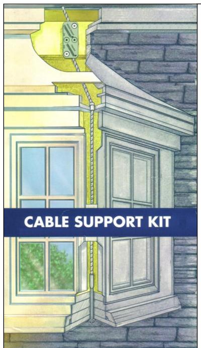
The Cable Support System, featuring the straight line clamp is used to secure the cable to the window. The unique design features a "no-slip" function that locks the cable in place. This is key!
