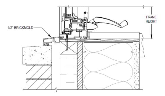
PROVIDE A CONTINUOUS BEAD OF SEALANT BEHIND THE NAILING FIN BEFORE SETTING THE UNIT IN PLACE OR SEAL FIN WITH WATER PROOF TAPE FILL VOIDS AROUND UNIT PERIMETER WITH INSULATION. DO NOT OVERFILL CAUSING UNIT TO BOW
