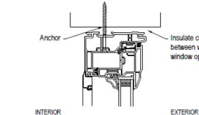
Insulate complete perimeter between window frame and window opening.
