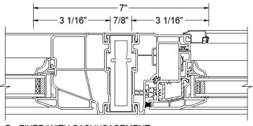
B - FIXED(WITH SASH)/CASEMENT MULLION 7/8" REINFORCEMENT DETAIL
