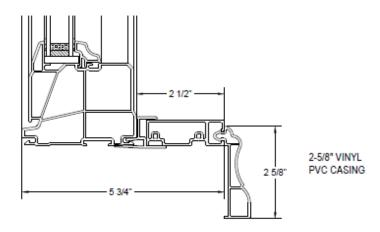
Note: The vinyl casings are joined by a Rosette/corner block on site. North Star will package separately to allow for window install
