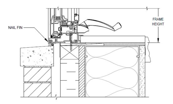
PROVIDE A CONTINUOUS BEAD OF SEALANT BEHIND THE NAILING FIN BEFORE SETTING THE UNIT IN PLACE OR SEAL FIN WITH WATER PROOF TAPE
