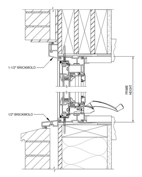
PROVIDE A CONTINUES BEAD OF SEALANT BEHIND THE NAILING FIN BEFORE SETTING THE UNIT IN PLACE AND SEAL FIN WITH WATER PROOF TAPE
