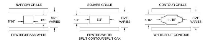
Note: For triple glazing, grilles are placed in exterior airspace
