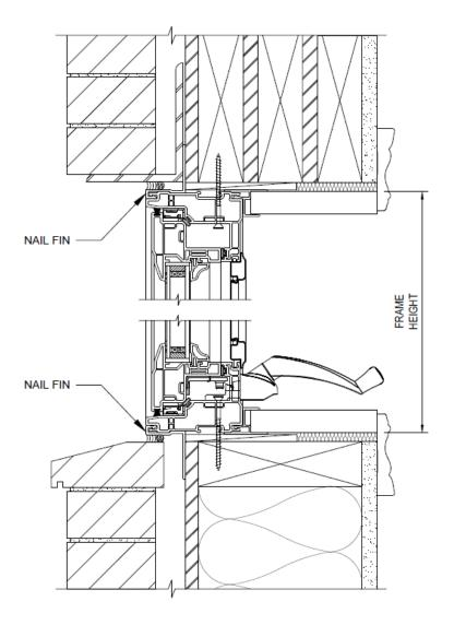
PROVIDE A CONTINUES BEAD OF SEALANT BEHIND THE NAILING FIN BEFORE SETTING THE UNIT IN PLACE AND SEAL FIN WITH WATER PROOF TAPE
