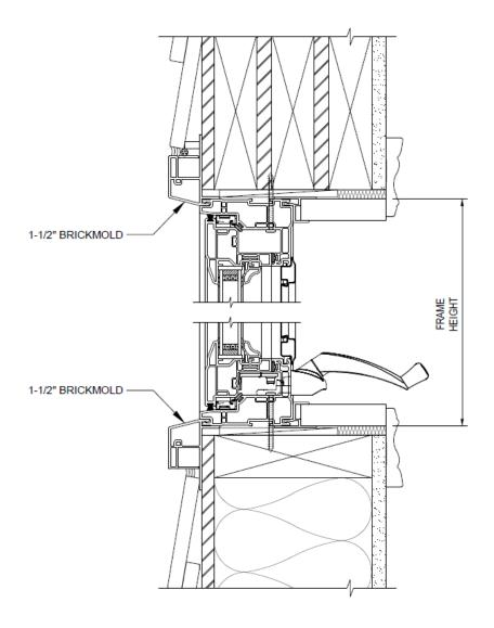
PROVIDE A CONTINUES BEAD OF SEALANT BEHIND THE NAILING FIN BEFORE SETTING THE UNIT IN PLACE AND SEAL FIN WITH WATER PROOF TAPE
