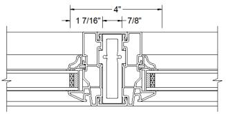
B - FIXED(NO SASH)/FIXED(NO SASH) MULLION 7/8" REINFORCEMENT DETAIL
