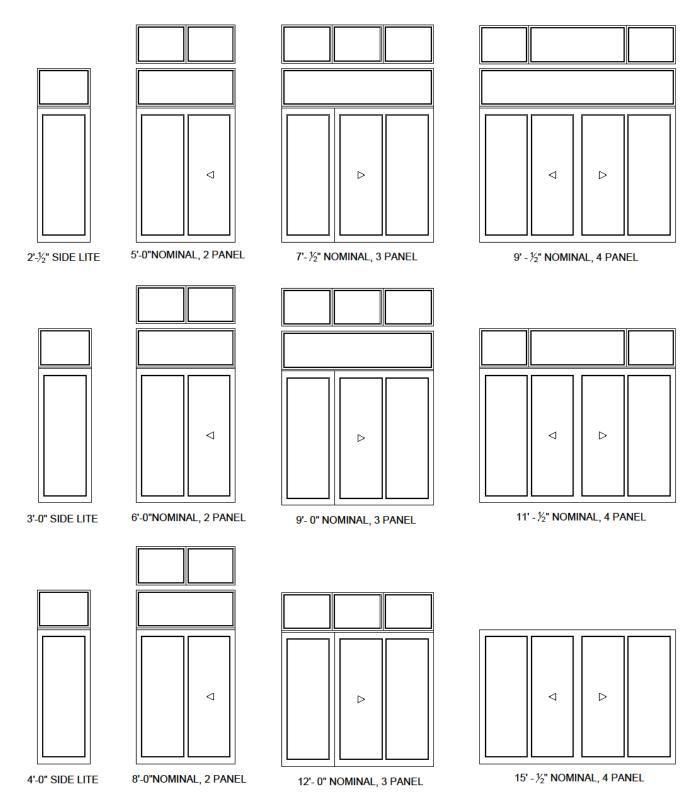
NOTE: 7/8" FIBREGLASS HORIZONTAL REINFORCEMENT IS INSTALLED BETWEEN PATIO DOOR AND TRANSOM
