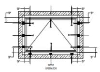
SHIMMING/ANCHOR LOCATIONS DEPENDING ON UNIT SIZE
