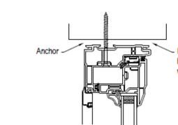
Insulate complete perimeter between window frame and window opening.
