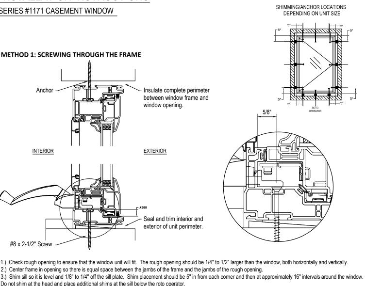
Check: Shims should be firm but not tight enough to cause the jambs to bow. Shims at the head should be loose to ensure window operation as the house settles. Check: level, plumb and squareness of frame and adjust shims if necessary
