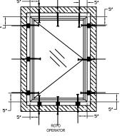
1.) Check rough opening to ensure that the window unit will fit. The rough opening should be 1/4" to 1/2" larger than the window, both horizontally and vertically.
